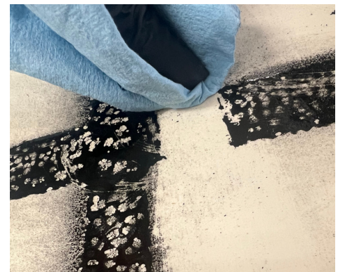
Remove with soap and water with light abrasion
