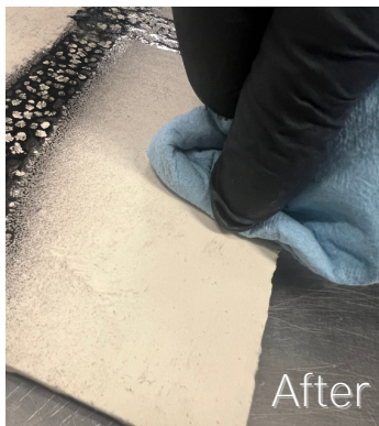
Creates a non-porous surface that resists graffiti adhesion
